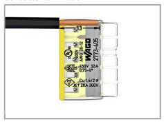
Strip solid or stranded conductor to 13 mm (0.51 inch)..
